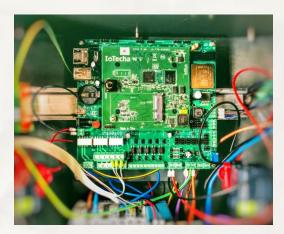
IoT.ON<sup>™</sup> DC EVSE Starter Kit is a complete ready-for-deployment EV charging controller for CCS DC EVSEs with out-of-the-box cloud integration.
